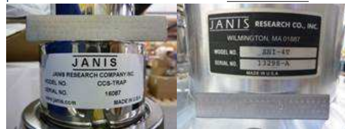
labels are usually near the evacuation valve or the instrumentation feedthrough
