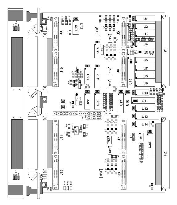
Figure 1 VIPC616 Assembly Drawing
