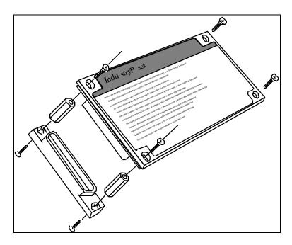
Figure 2 IndustryPack Installation
