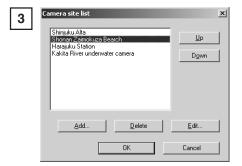
While a camera site is selected, you can move it to a different position in the list by clicking the Up or Down button. This order is reflected in the list displayed in the Site Selection dialog box.
