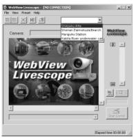
Select the connection target from the site selection box. The camera servers displayed here are sites that were registered by selecting "Add to camera site list (see p. 28)" when a connection was made by specifying a connection target, or registered using the "Register connected site button (see p. 38)".
