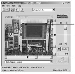
By clicking a point on the video, you can move the center of the camera to that point.
