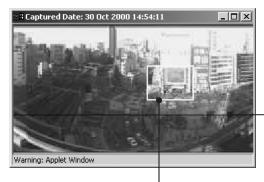
The black frame indicates the range of movement for the camera center. The camera center cannot be moved outside this frame.
