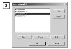
While a relay server is selected, you can move it to a different position in the list by clicking the Up or Down button. This order is reflected in the list displayed in the connection dialog box.
