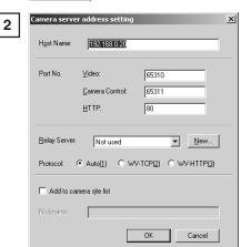
A dialog box for specifying a connection target appears. Enter each item and click OK to make a connection to the camera server.
