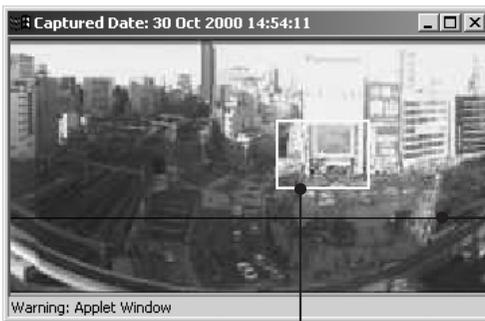
The black frame indicates the range of movement for the camera center. The camera center cannot be moved outside this frame.
