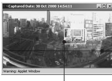
The black frame indicates the range of movement for the camera center. The camera center cannot be moved outside this frame.
