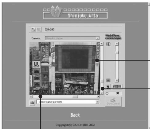
By clicking a point on the video, you can move the center of the camera to that point.
