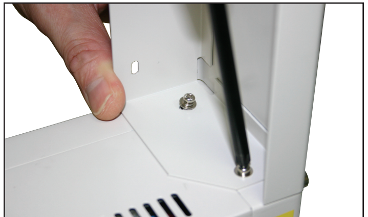
Step-9 Attach rack-mount extension panel for full rack installation
