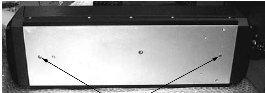
DOWEL PIN HOLES
