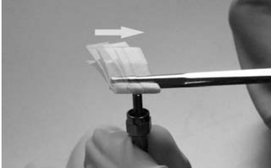
Figure 6-16. Placement and Movement of the Folded Tissue Against the Fiber Optic Surface
