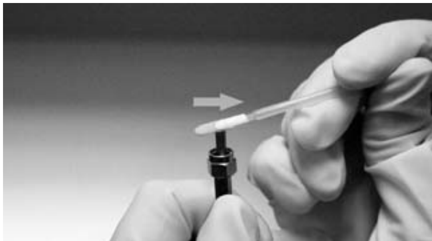
Figure 6-12. Placement and Movement of the Swab Against the Fiber Optic Surface
