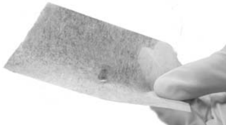
Figure 6-7. Methanol Drop on Lens Tissue
