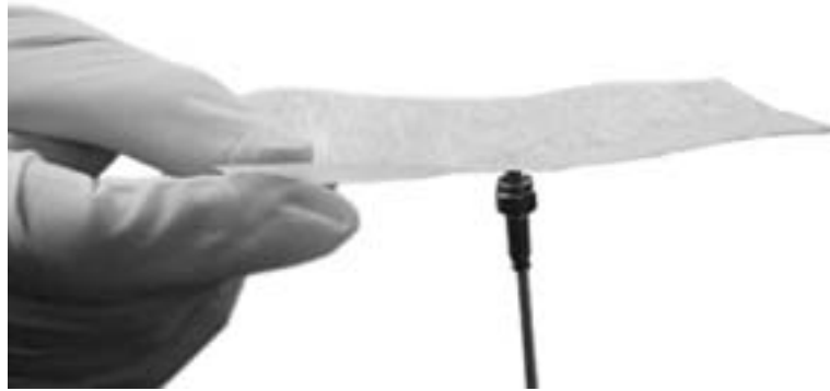
Figure 6-8. Placement of the Fiber Optic Against the Lens Tissue
