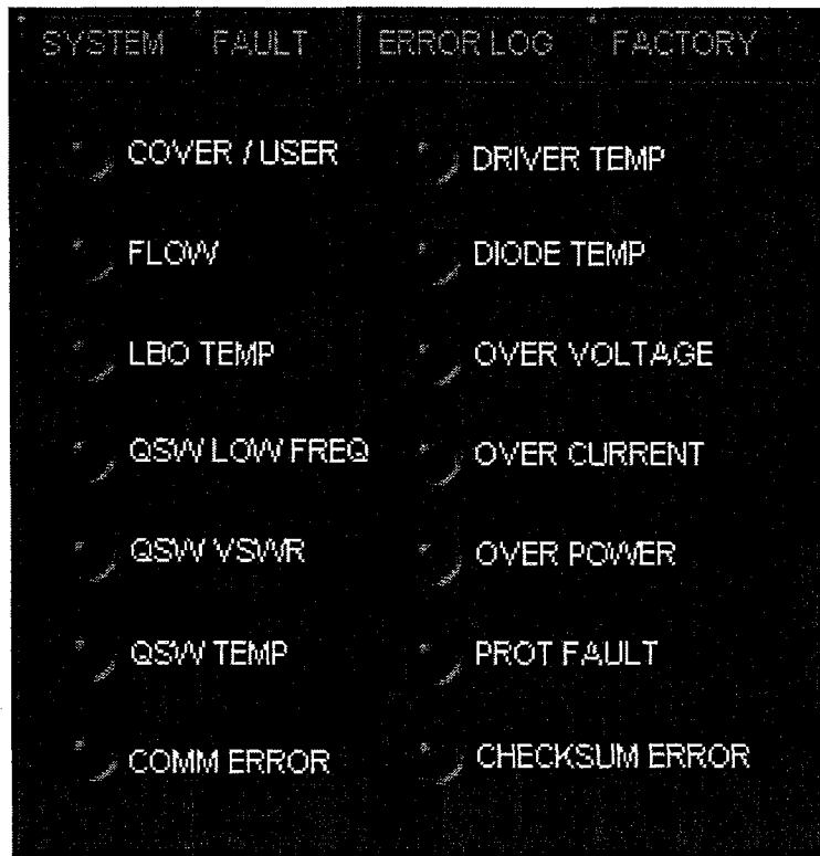
Figure 3.6: Control Software FAULT Panel.
