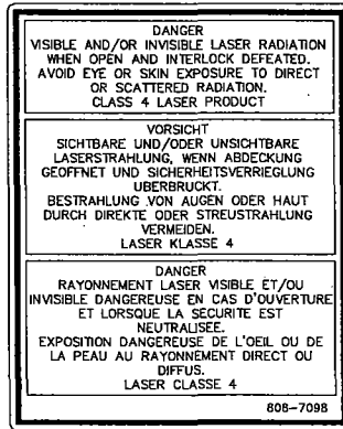
CE WARNING LABEL, INTERLOCK DEFEATED (9)
