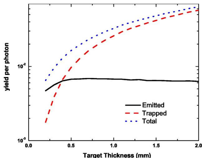
FIG. 3. (Color online) Total, trapped, and emitted positron yields per photon as functions of target length by EGS4 Monte Carlo simulation. The calculation is for the spectrum in Fig. 1(a).
