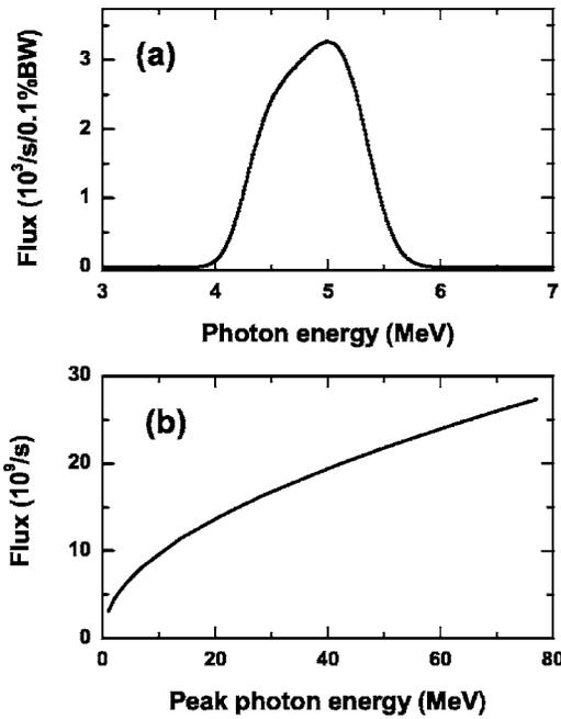
FIG. 1. (a) A  $\gamma$ -ray spectrum peaked at 5 MeV. (b) The total flux as a function of the peak photon energy. An acceptance angle of  $1/\gamma$  is used in the calculation, where  $\gamma$  is the relativistic factor of the beam. The crossing angle is 0.13 rad. In (b), the peak photon energy is tuned by changing the interaction angle between the laser and the electron beam. Here a laser repetition rate of 4 kHz and an optical cavity with a quality factor of 1000 at 6.52 MHz are considered.
