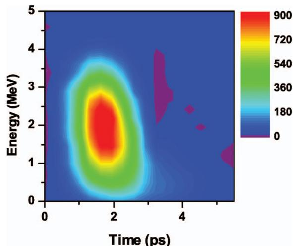
FIG. 4. (Color) Positron spectrum as a function of time, calculated by EGS4 Monte Carlo simulation. The calculation is for the spectrum in Fig. 1(a) with a 1 mm tungsten target. The intensity scale is relative.
