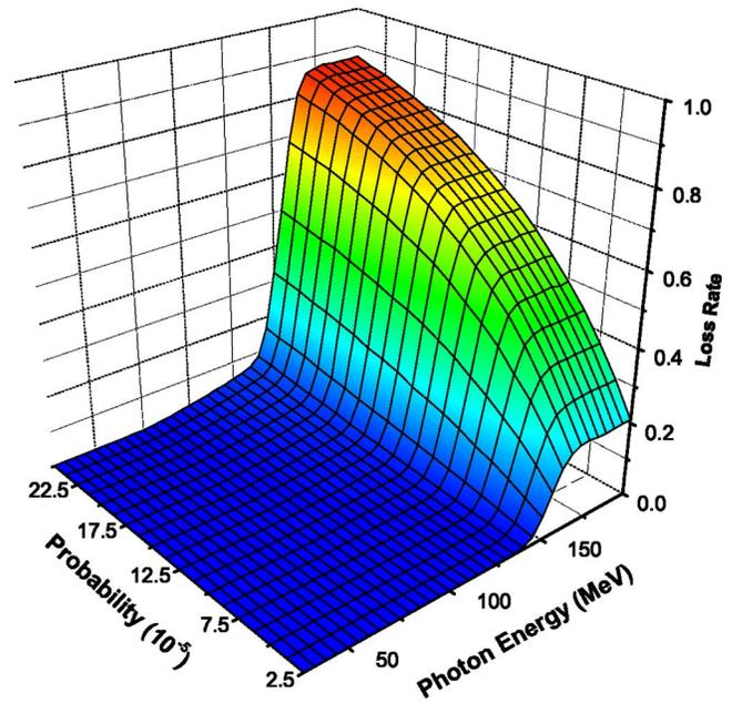
FIG. 2. (Color online) Electron loss as a function of  $\gamma$ -ray photon energy and the radiation probability per turn. Note the thresholdlike behavior at photon energy of about 140 MeV.
