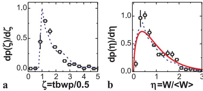
**FIGURE 4** Probability distributions of (a) the normalized rms time-bandwidth product,  $tbwp/0.5 = 2\sigma_t\sigma_\omega$ , where 0.5 is the transform-limited value, and (b) the pulse energy. Symbols: experiment; dashed lines: simulation; solid line: theory
