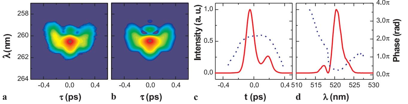
**FIGURE 1** An example of a single-shot FROG measurement. (a) Raw data, (b) reconstructed image from FROG algorithm, (c) time-domain intensity and phase evolution, and (d) frequency-domain intensity and phase evolution. *Solid lines: intensity; dashed lines: phase*
